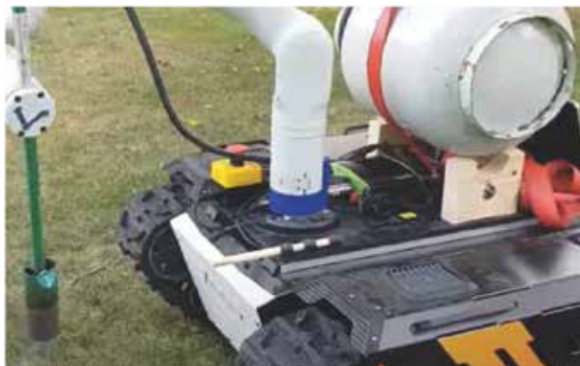
Slika 7. Robot za suzbijanje korova plamenom Ultimate Weed Killing Robot Figure 7. Robot for weed control by flame Ultimate Weed Killing Robot Izvor/Source: https://hackaday.io/project/181763-ai-powered-weed-killing-robot
